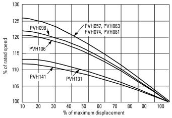
Note: Speeds at 10% displacement represent maximums at load-sense standby condition. These speeds must be reduced to rated speeds at 100% displacement before leaving standby condition, or pump damage may result.
