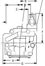
Right hand rotation, pressure compensated and torque limit model
