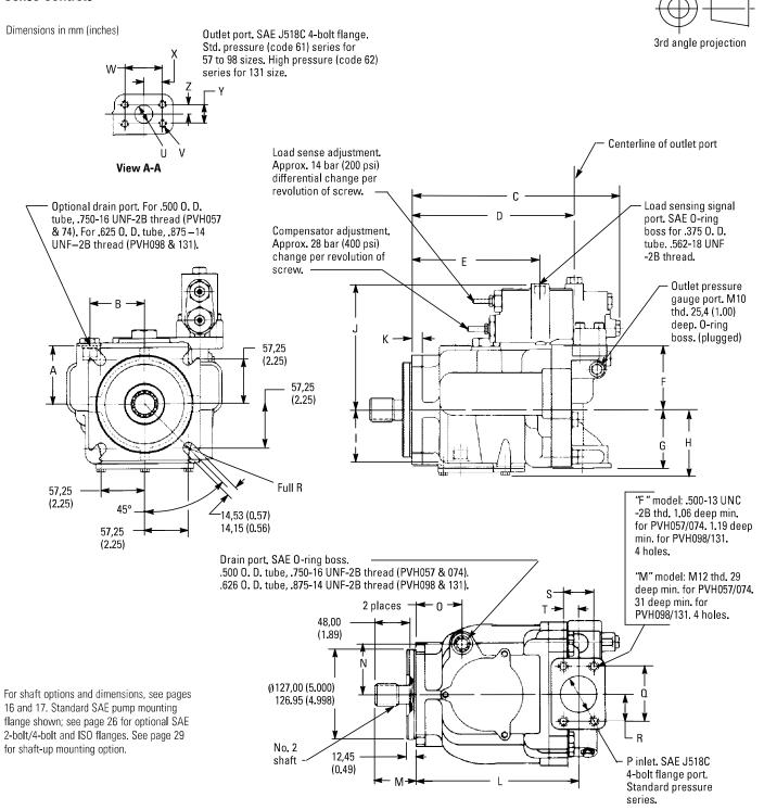
Basic Pump with Pressure Compensator and Load Sense Controls
