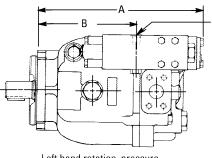
Left hand rotation, pressure compensated with load sense and torque limit model
