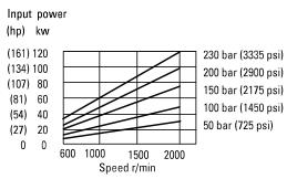
Performance data is typical with SAE 10W anti-wear hydraulic oil at 50°C (120°F) and at zero pump inlet pressure, except where otherwise indicated.
